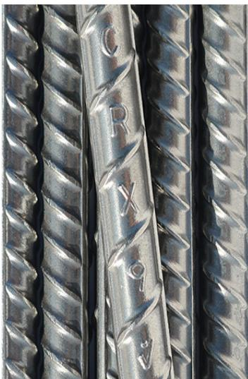
This guide includes a discussion of the material characteristics of Grade 100 (690) ASTM A1035/A1035M (CS) deformed steel bars and recommends design criteria for beams, columns, slab, systems, walls, and footings for Seismic Design Category (SDC) A, B, or C, and for structural components not designated as part of the seismic-force-resisting system for SDC D, E, or F.
