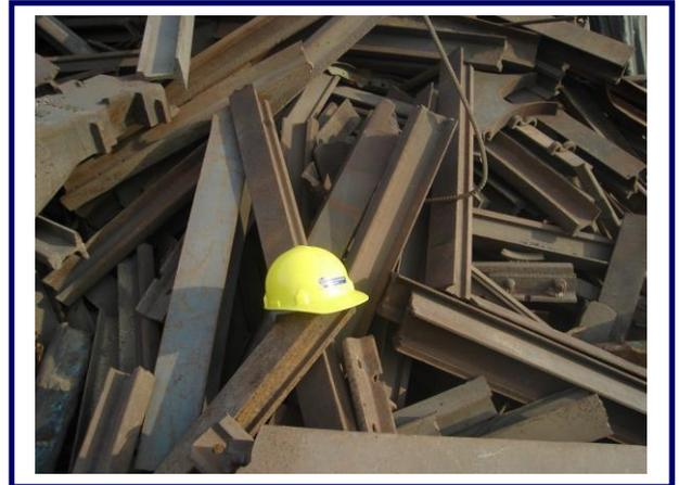
**DESCRIPTION:** Cut allow-free railroad scrap to include track, spikes, tie plates, wheels, drawbars, knuckles, etc. Car sides are specifically excluded. Wheels must be pressed or cut off axles or axles cut flush with wheels.
