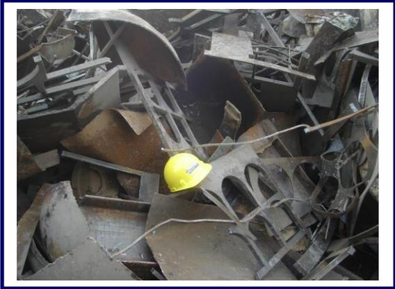
**DESCRIPTION:** Very dense, clean, new or obsolete steel plates (includes torch cut plate or skeleton plate), structural shapes or crop ends. Should be free of non-ferrous metals and other contaminants.
