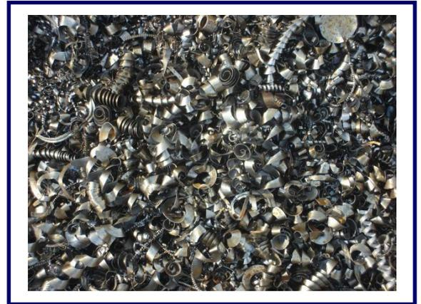
**DESCRIPTION:** Clean, dense steel turnings from fresh production. May not be **springy, bushy, tangled or matted**. No long, stringy pieces. Turnings that are not easily handled by a magnet will be rejected.
