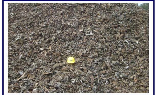
**DESCRIPTION:** Extremely dense, clean, homogenous iron and steel scrap, magnetically separated originating from automobiles, unprepared #1 and #2 steel and miscellaneous baling and sheet scrap, essentially free of non-metallic and non-ferrous material. Automotive scrap used to produce shredded scrap must be purchased ONLY from suppliers that are active members of an EPA approved mercury switch removal program such as National Vehicle Switch Removal Program (NVMSRP).
