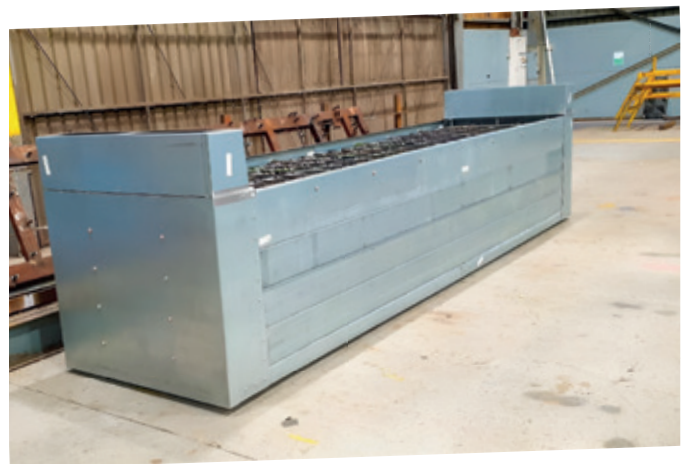
Figure 2. Completed single lane pier cap in the factory.
