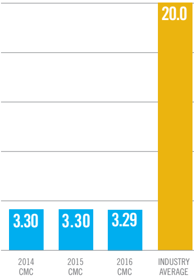
Energy Intensity (GJ/Ton) Required to Produce CMC Products (2014, 2015, 2016) vs. Global Industry Average Products (2016) (as reported by Worldsteel Association)
