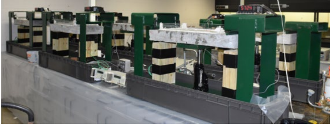
Figure 11 Typical Setup of Accelerated Corrosion Tests
