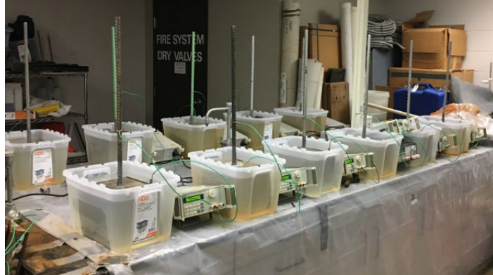
Figure 4 Test Setup of Pullout Specimens Subjected to Accelerated Corrosion
